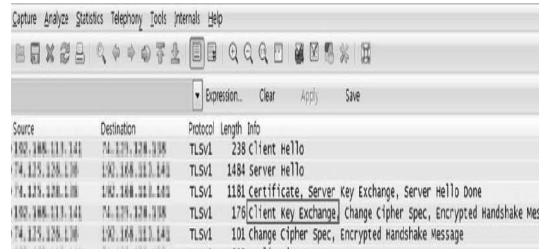
Fig.7. Captured Packets of SSL Handshake Protocol
