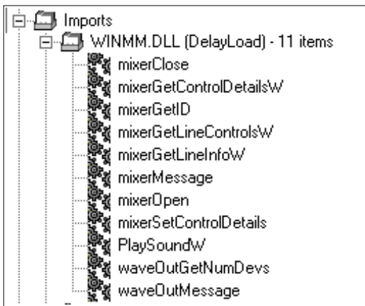
Fig. 3. The Import section information of 'explorer.exe' which embeds 'winmm.dll'
