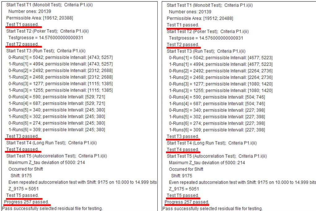
Fig. 13. For 40,000 bits sample sequence, compare results for LRNG source when significance level  $10^{-4}$ (left) and  $10^{-6}$ (right)
