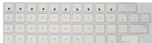
Fig. 1. Anti-screenshot virtual keyboard. Keys within the row are replaced by special character.
