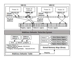
Fig. 3. Overall architecture for malicious behavior detection in cloud platform
