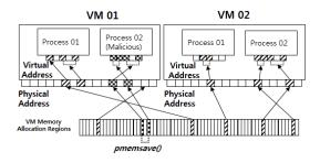
Fig. 1. Partial memory dump for cloud instance using 'pmemsave'
