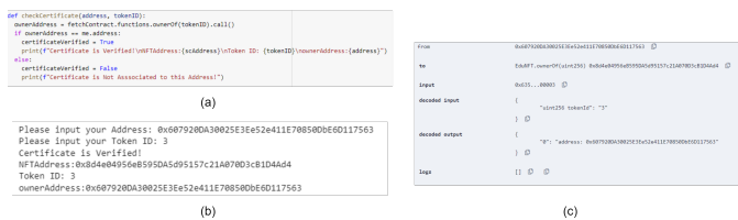
Fig. 2: Validation of the execution of certificate management: (a) pseudocode implementation in Python, (b) Python execution result on certificate verification, and (c) Smart contract execution results of getting the owner address of a Token
