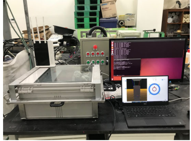
(b) Automatic lifting cable control system
