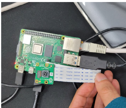
Fig. 3. Surveillance camera module based on the Raspberry Pi 4.
