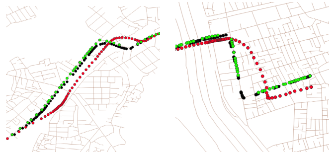
Fig. 2. Prediction results at intersections, where green, red and black dots are the proposed, vanilla LSTM and the actual trajectory result, respectively.
