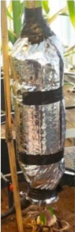
a) Sap flow sensor for small stems at USDA's farm
