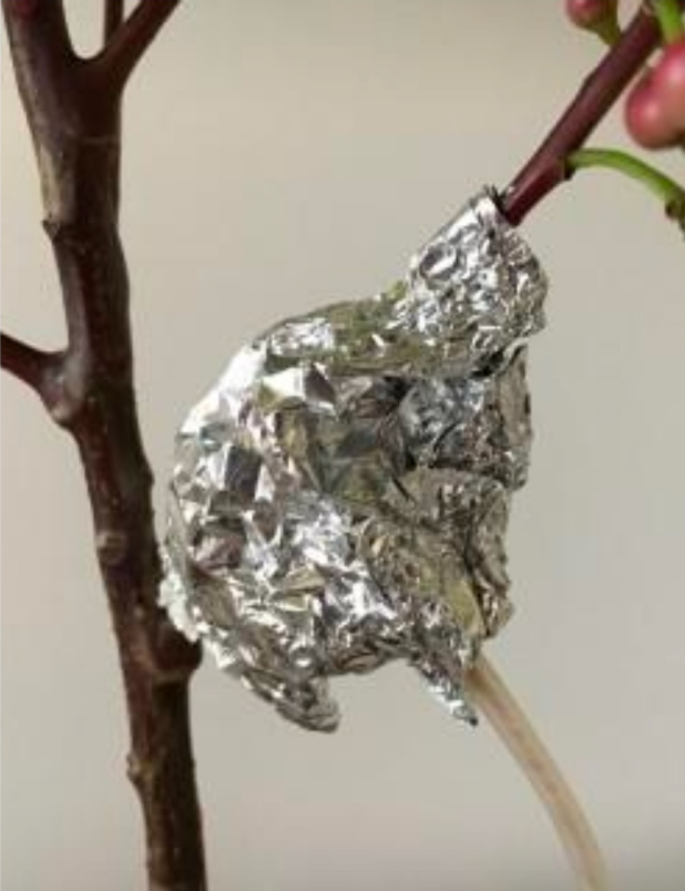
a) Sap flow sensor for small stems at USDA's farm
